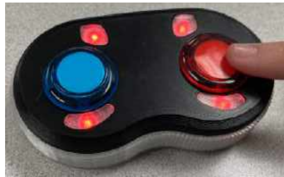
Figure 1: The Sistance device with the red input button activated - the red LEDs, buzzer and vibrational motor running.
