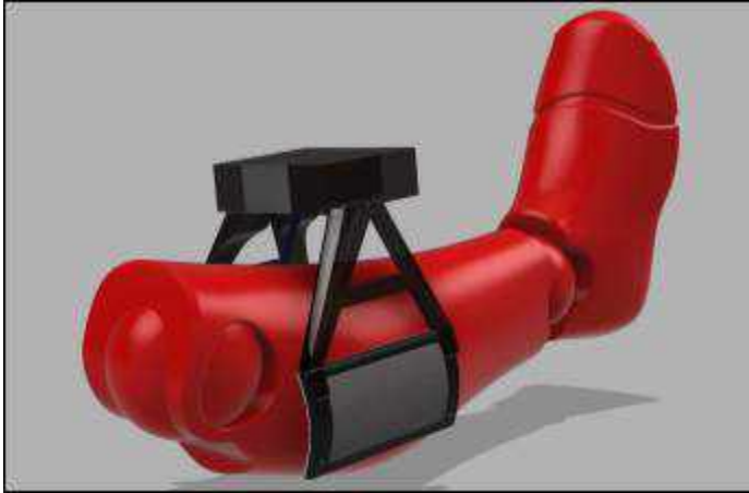
Figure 1: Render of device from Fusion360 displaying lateral clamp placement and displacement probe tip placement on model right leg.
