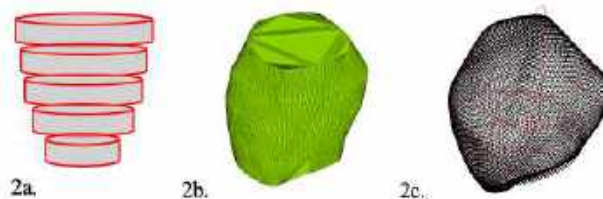
Fig. 2 compared methods for volume calculation: (a) Simpson’s Disc Summation; (b) SA \alpha -shape estimation; (c) LA + SA \alpha -shape estimation
