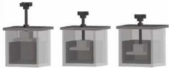
Figure 1. CAD model illustrating the incremental compression device at various levels of applied compression.
