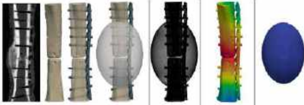
Figure 2: Workflow showing model creation, meshing, simulation and submodeling (blue zone) to measure interfragmentary strain.
