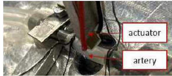
Figure 1: OCE measurement of ACA cannulated on a custom device and pressurized up to 120 mmHg.
