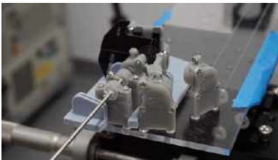
Figure 3. This photo contains the main stage resin optomechanics slotted into our acrylic laser cut panel/stage for a preliminary prototype. In this photo, we have placed the device's true lenses and mirrors into the optic holders and began alignment with a collimated beam.
