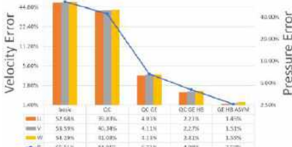
Figure 2: L2 norm velocities and pressure errors of the vanilla PINN and PINN in combinations with various strategies.
