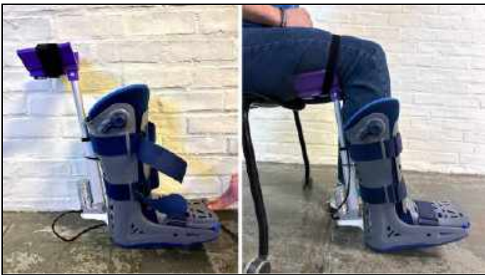
Figure 1: Side view of the device attached to a patient's leg
