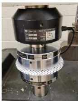
Figure 3: Engineered foam undergoing compression testing.
