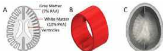
Figure 1: Cranial phantom outline (a), 3D-printed skull (b), cranial phantom in skull (c), adapted from Knutsen, et al., 2023.
