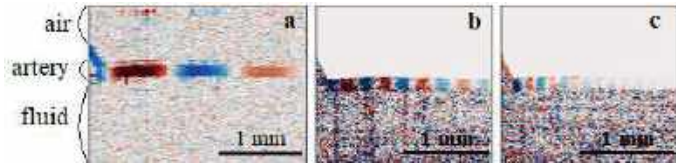
Figure 2: Displacement maps at frequencies of (a) 10 kHz, (b) 30 kHz, (c) 50 kHz in an ACA wall pressurized to 80 mmHg.
