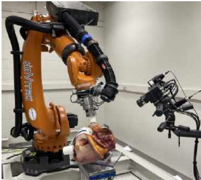
Figure 2: Experimental set-up showing sacrum fixed to pedestal and right femur fixed to robotic arm with optical metrology cameras viewing.
