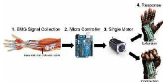
Figure 2: Summary Diagram. The EMG signal is taken from the forearm, processed by an Arduino Uno and sent to the motor which then activates a contraction or releases to allow extension.
