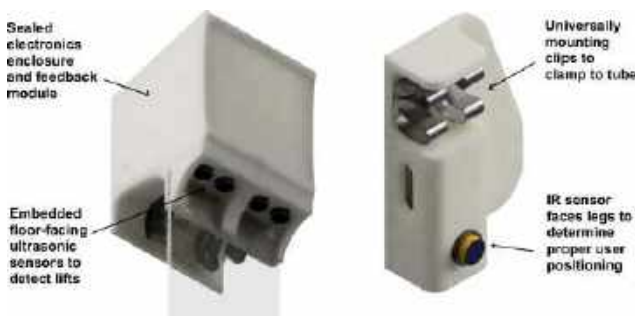
Figure 3: Isolated Views of Design Modules
