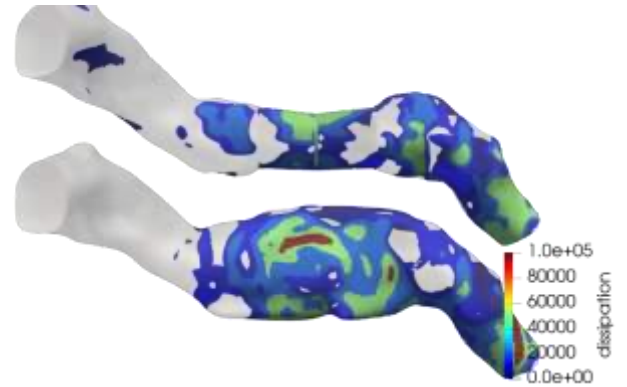
Figure 2. Dissipation rate (W/m 3 ) in the t-junction and y-graft geometries, posterior wall visible.
