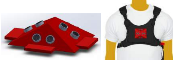
Figure 1. Trimetric View of 3D Printed Case for Sensors (left) and Device Worn on Chest (right)
