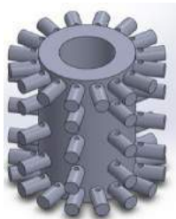
Figure 3: CAD model of metal jig designed for braiding the valve stent
