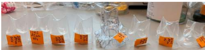
Figure 2: From left to right, LLDPE films that were thermoformed under different durations of 50, 40, 30, 20, 19, 18, 15, and 10 seconds.
