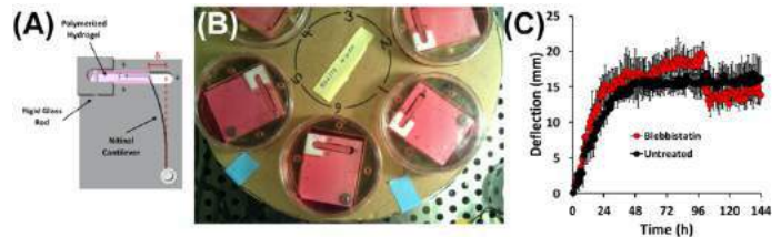
Fig. 2: (A) Schematic showing the main components of the force bioreactor and measurement of the amount of wire deflection, \delta . (B) An overhead camera images each of 6 bioreactors every hour. The bioreactors slowly rotate under the camera via a turntable. (C) Gel compaction and wire deflection generally reach equilibrium after 48 hours. Addition of blebbistatin in DMSO temporarily reduced cell traction forces by ~ 30%.
