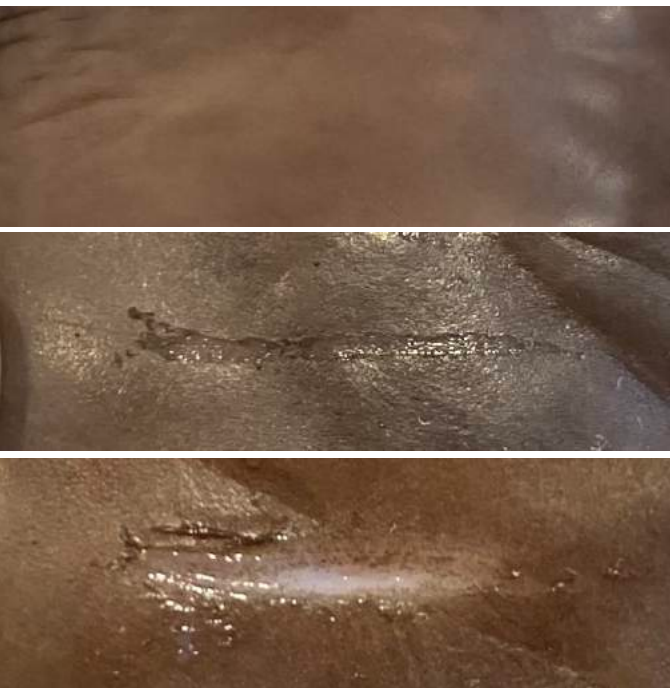
Figure 2: The fetal bovine skin surrogate showing no injury in test 12-I (top), a minor abrasion in test 14-I (middle), and a minor laceration in test 16-I (bottom).
