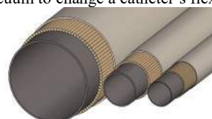
Figure 1: CAD model of the layered MultiFlex catheter design.
