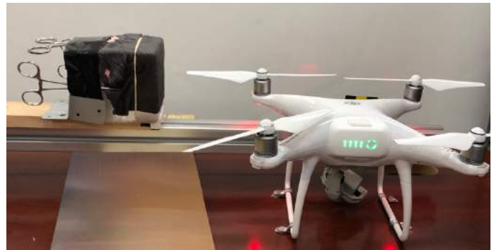
Figure 1: Testing configuration with fetal bovine skin mounted on a slide moved into the Phantom 4 blade.
