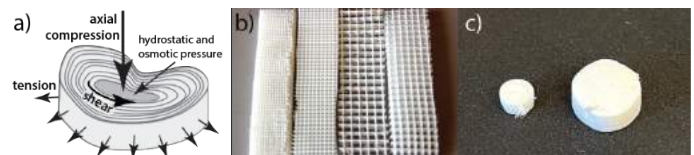
Figure 1: a) Schematic of IVD loading, b) 3D printed FPLA meshes, c) 3D printed FPLA IVD disks for rat and 2X scaled up dimensions.
