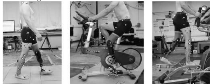
Figure 1. Experimental setups for gait (left), cycling (middle), and elliptical (right) experiments for control and amputee participants.
