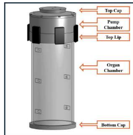
Figure 1: VOPS Device Design Components
