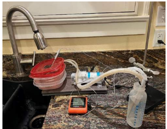
Figure 1. Warming technology circulates milk via a pump from a bottle directly into a copper coil which is submerged in a bath containing hot water from the faucet. Bottle warming takes about 15 s to warm 8 oz milk bottle from refrigerator temperatures (4 °C) to body temperature (37 °C).
