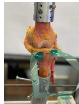
Figure 1: MTS 30/G Machine with Tekscan sensors in knee.
