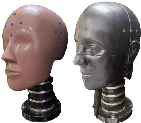
Figure 1. Experimental setup of the Hybrid III headform (left) and the NOCSAE headform (right), which were each marked with 5 frontal and 5 temporal targets to impact with the tip of the impact hammer.
