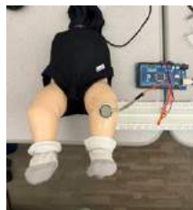
Figure 2: Hippy Baby Instrumented with a FSR
