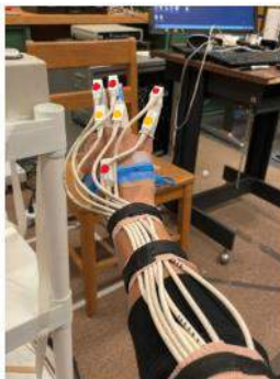
Figure 1. Sensors were affixed the palm and proximal and distal phalanx of each finger. The goal of the research was to determine if the distal phalanx orientation could predict the proximal phalanx orientation for an array of motions and orientations.
