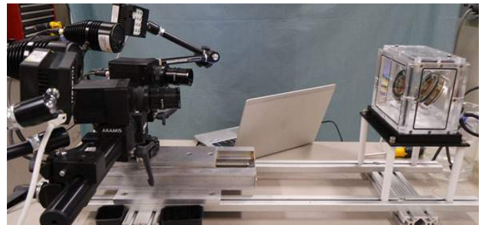
Figure 1: Test set up with camera mount on left atop test rack and acrylic chamber on right equipped with angled mount.
