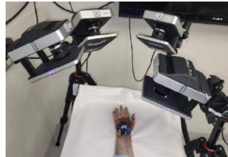
Figure 1: Four Vicor cameras recording marker positions at each pressure level.
