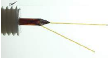
Figure 3: Side and center microneedle deployment distance from the main cannula controlled by the actuation block, not pictured.
