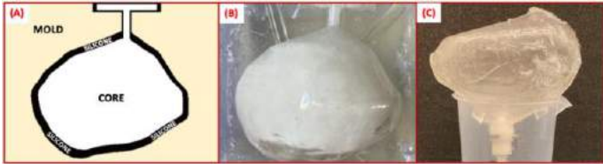
Figure 1: (A) Schematic of in-vitro fabrication method used to make physical model. (B) Silicone model before dissolving bladder core. (C) MRI- and PIV-compatible hollow bladder flow model (note the model in the anatomical standing position).
