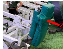
Figure 1. Mounting of the force plate with green blocking pad secured. Z-direction was labeled to show the direction of recorded force.
