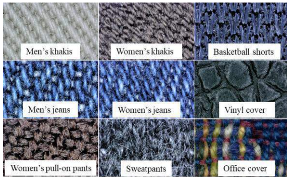
Figure 2. The fabric structures of all the pant fabrics and seat covers under 50x magnification.
