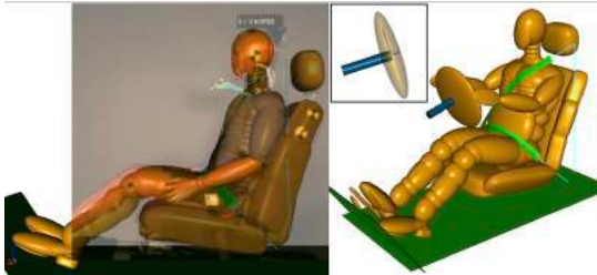
Figure 1: MADYMO build position matched to IHS SER01040 and steering wheel loadcell orientation.
